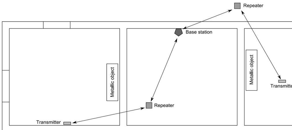
In multi-storey buildings, it is recommended to use a central repeater to get sufficient radio coverage.
